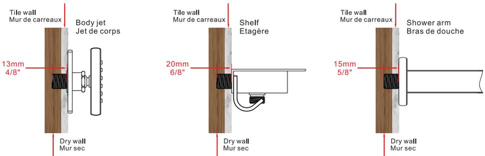
The thickness of the tile must be calculated for installation.
