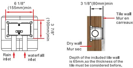
⚠ If the Inwall box is embedded too deep, the shower head will not be installed properly and it will cause water leakage and sag problems. Please pay attention to the installation depth.
