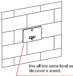
4. Install Shower head body. First remove box cover and plug, screw Two water inlets into inwall box with
