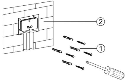
3. Remain inwall box in same level as wall after seal the tile and cover exceed wall.
