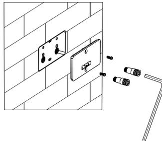
5. Install Flange as picture. Caution: horizontal and vertical position of shower head before wall seal. Install the screw to avoid any trouble of repair after wall seal.
