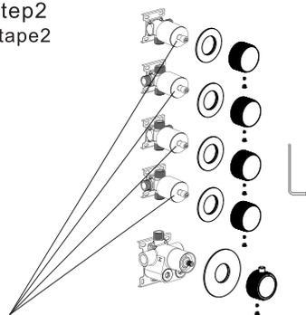
Do not remove the white wear ring; otherwise, the handwheel will be damaged.
