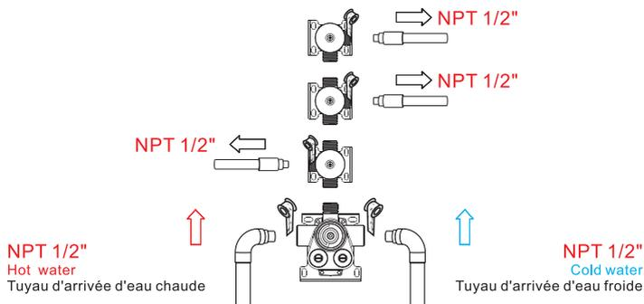
1. As shown in the figure, the inlet and outlet pipes are pre-buried. Please pay attention to the correct direction of installing the pre-buried main body.
