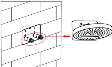
6. Twist the screw with a screwdriver into the embedded box and install it
