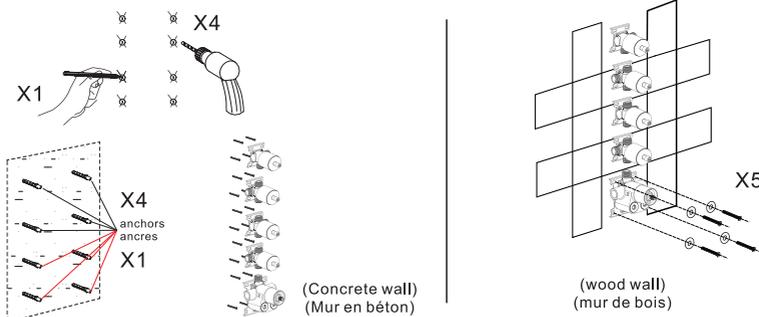
1. Make marks according to the size of the main body valve, and then drill anchors into the wall (concrete wall).
