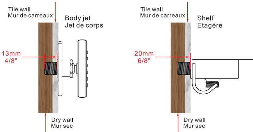
The thickness of the tile must be calculated for installation.
