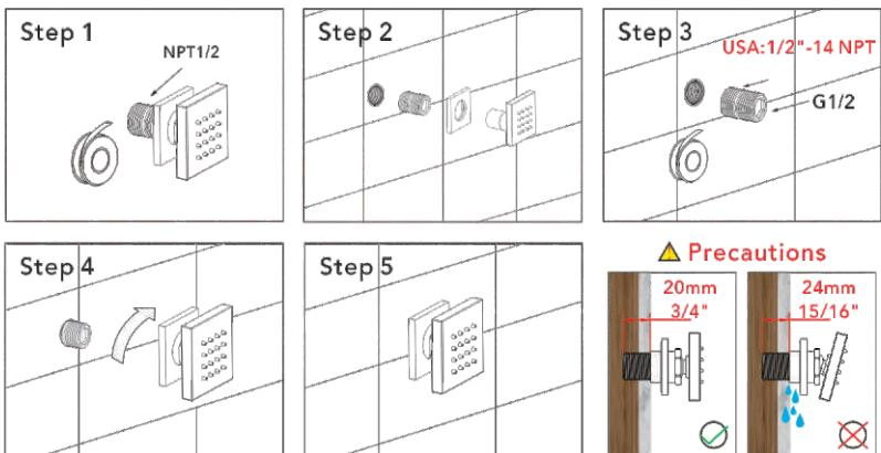
Step 1: Ensure that the threaded pipe and the raw material tape are of matching sizes to avoid misalignment when screwing into the wall.
