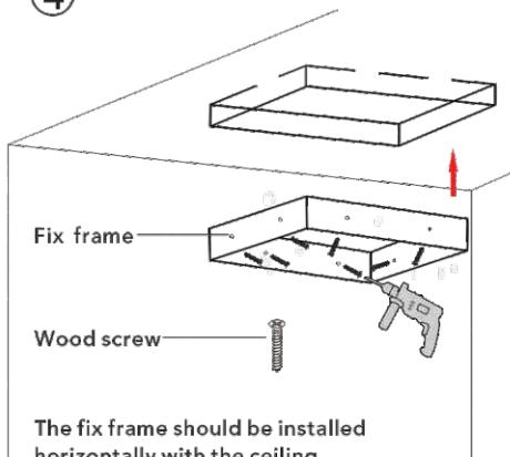
The fix frame should be installed horizontally with the ceiling.
