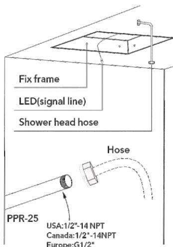
Connect one end of the corrugated pipe to the embedded PPR water pipe and the other end to the water inlet pipe on the back of the shower head.
