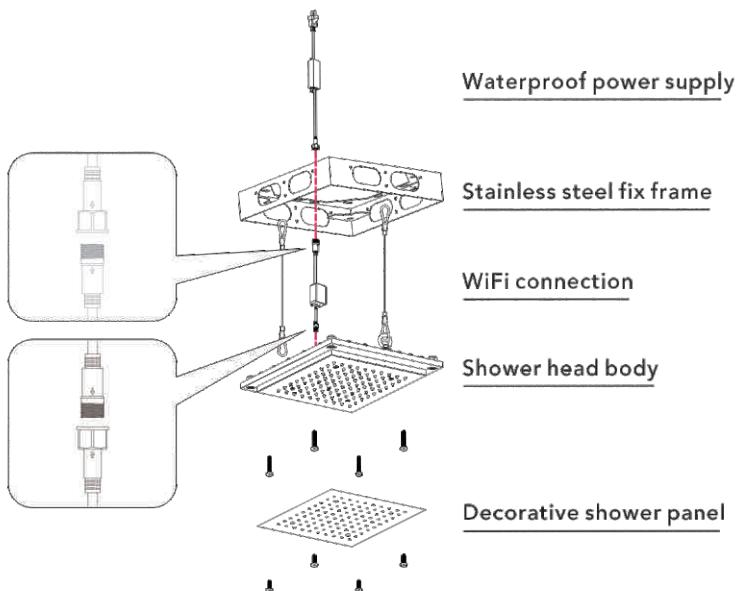
According to the mark (Remove/Install) on the top of the shower head panel, unscrew the decorative shower panel, shower head body, and fix frame respectively.
