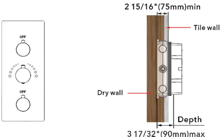
Notice: 1. The installation depth of the main body should be no less than 2 15/16" (75mm) and no more than 3 17/32" (90mm), including the thickness of the tile. Otherwise, the deck plate cannot be installed.
