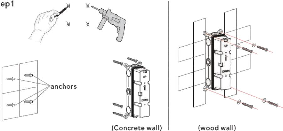
1. Make marks according to the size of the main body valve, and then drill anchors into the wall (concrete wall).
