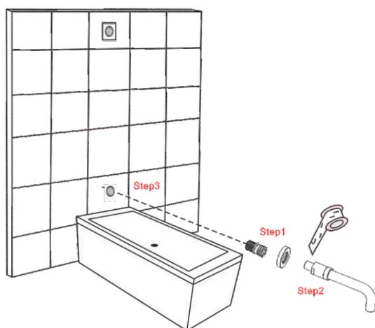
**Step1:** Connect the copper connector to the bathtub spout and wrap it with waterproof tape.
