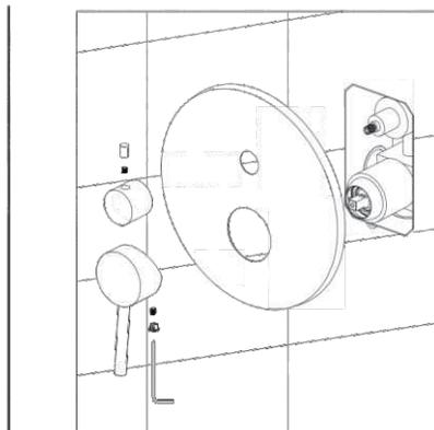
1. Make marks according to the dimensions of the main body valve, then drill anchors into the wall (for a concrete wall).
