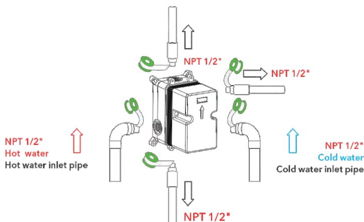
1. As shown in the figure, the inlet and outlet pipes are pre-buried. Please pay attention to the correct direction when installing the pre-buried main body.
